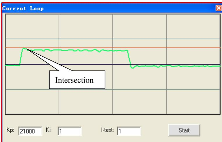
**Step 4:** Now the **K<sub>p</sub>** is relatively good enough. But there is still distance between the green curve and the red curve when we use the mouse to zoom in the green curve. So we need to introduce **K<sub>i</sub>** to reduce the distance or steady error at the constant part. It follows the same procedure as **K<sub>p</sub>**. High **K<sub>i</sub>** causes big vibration, system lag and makes the performance worse. The following figures show how to tune the **K<sub>i</sub>**.
