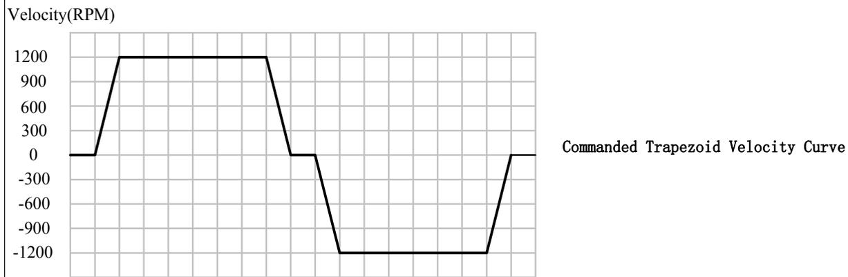
Our purpose is to get the highest system stiffness but lower motor noise. The actual measured velocity should be similar as the commanded velocity curve. However, sometimes we need to trade off between high stiffness and low motor noise because high proportional gain leads to big overshoot and vibration. In this example, we start with small proportional gain then increase it. We will stop increasing when the motor noise can not be accepted. The tuning procedure is shown as follows:
